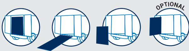
**DEPLOYMENT:** The WM Light is extremely lightweight, using both spring and gas strut assistance. An external swivel kit is supplied on request, making it possible to gain access to the van like a second door.
