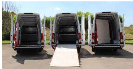
Shot-blasted non-slip aluminium surface
