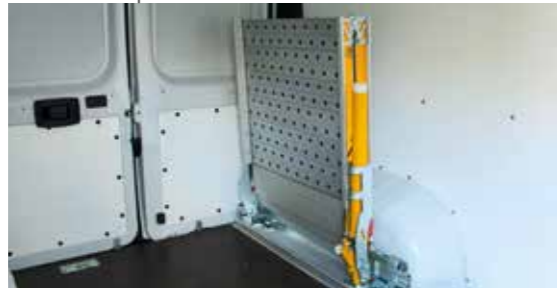
Anti-slip anodised aluminium perforated platform
