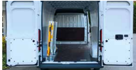
Flexible contact plate to the van floor
